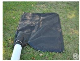
GS Dewatering Bags are an economical filtration solution designed to help filter silt and sediment out of water. GS Dewatering Bags remove silt, sand, and other debris from pumped water on construction sites, ponds, dredging locations and more. These Bags are designed using a heavy GSM Non-Woven Needle Punched Geo Textile Fabric, generally 300 GSM / 400 GSM.
